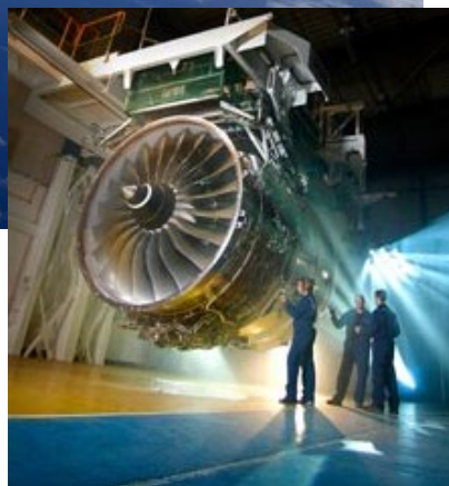
The new Boeing 787 Dreamliner aircraft and its Rolls Royce engine used titanium to reduce its own weight for fuel efficiency purposes
