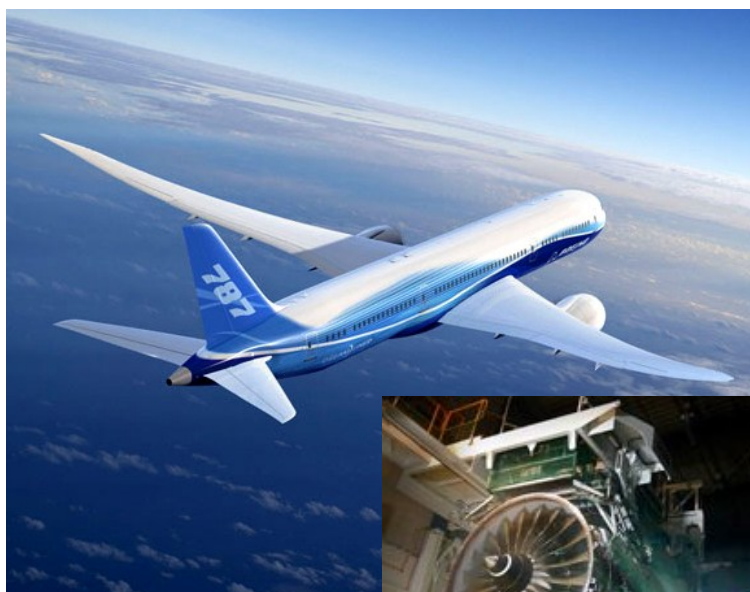
The new Boeing 787 Dreamliner aircraft and its Rolls Royce engine used titanium to reduce its own weight for fuel efficiency purposes
